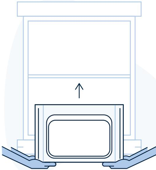
Together with your helper, lift the assembled AC into the window frame.
