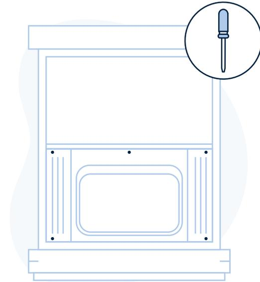
**Secure the AC using the included 1/2 inch screws.**
