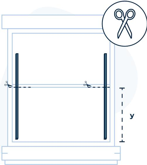
**Cut the non-adhesive foam to the height of the bottom half of your window.**
