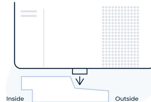
Properly position the bottom bar **BEHIND** the inside window sill.
