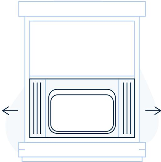
**Use the side panels to fit the AC to the window.**
