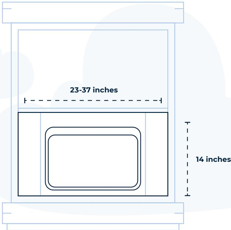
The medium size (8K BTU) Windmill AC is designed for windows that slide up and down (double-hung windows) with a width of 23-37 inches and a vertical opening of at least 14 inches.
